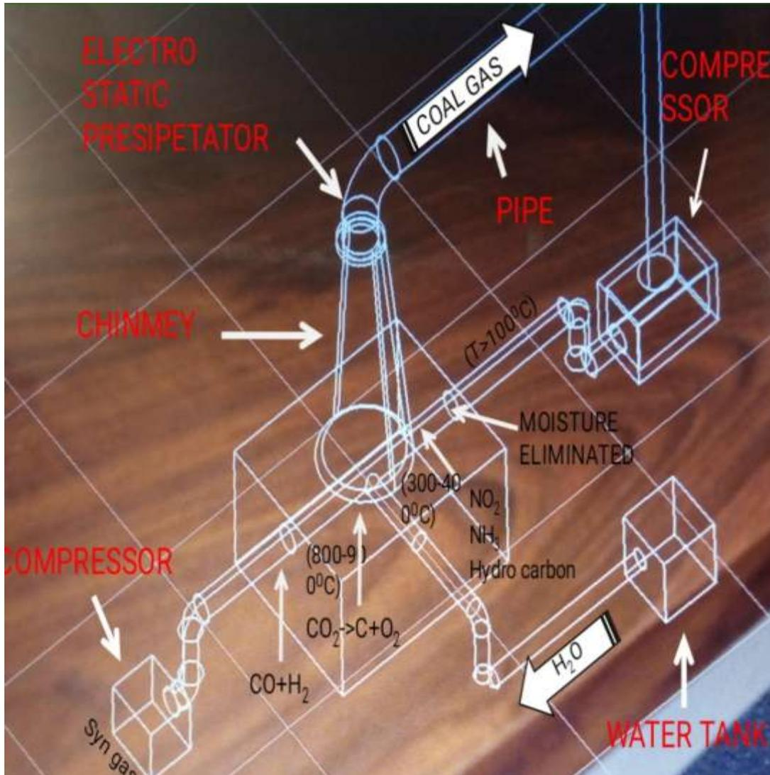
Fig. 5 ( Complete process of reducing the coal gases) made by self on catia
