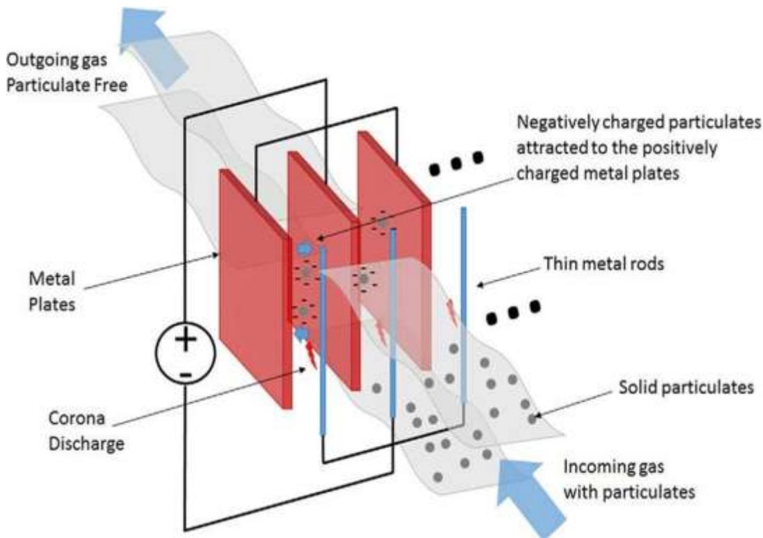
Fig. 2 ( Electrostatic precipitation) [www.sorcedata.com](http://www.sorcedata.com): data
